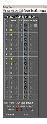
DX-PC For View provides a status display, remote setup, system log and event log view of the connected remote site in real-time. To display a status of the remote site, select a camera or a site from the Remote Site list and drag it to the Status View panel. You can also select **Connect Status** from the popup menu displayed by clicking the right mouse button after selecting the site from the Remote Site list.
